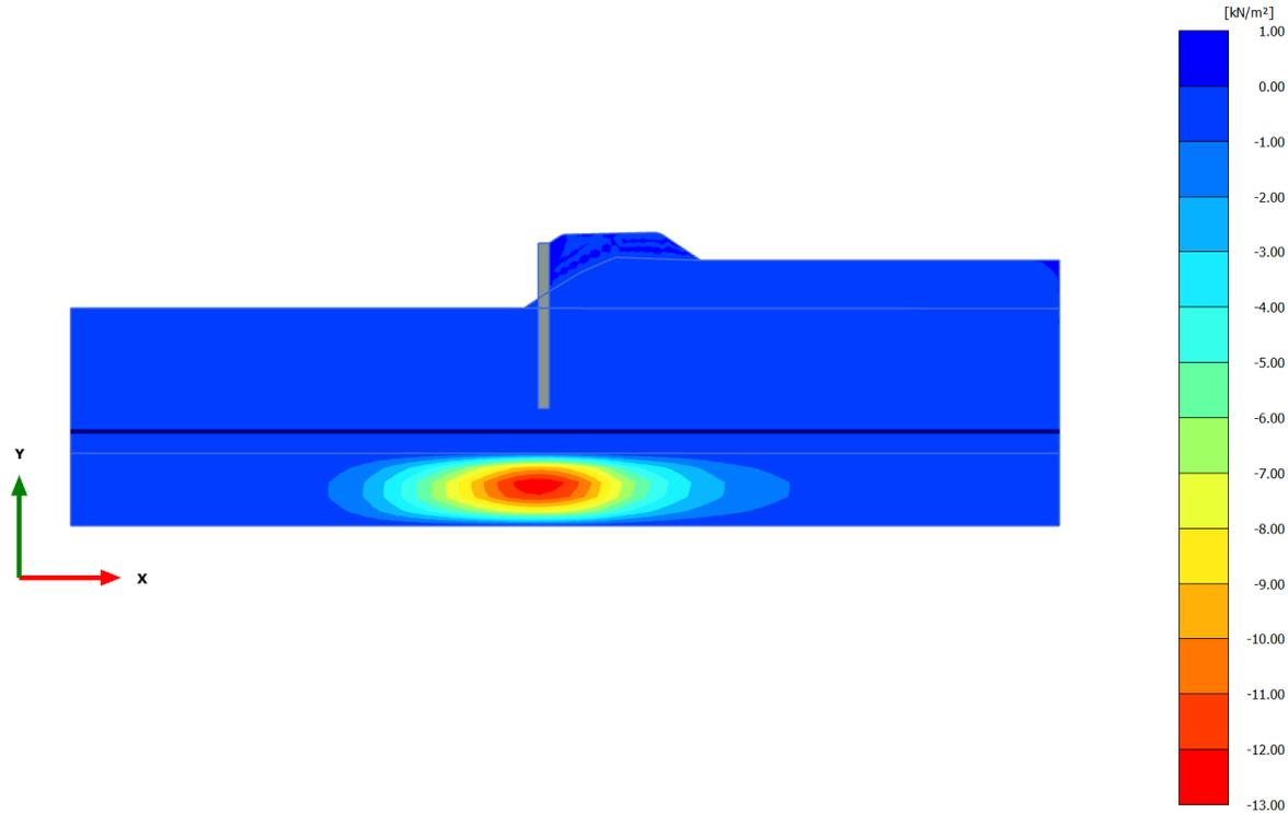
Excess pore pressures  $p_{\text{excess}}$  (scaled up 0.500 times) (Pressure = negative) (Time 330.0 day)
