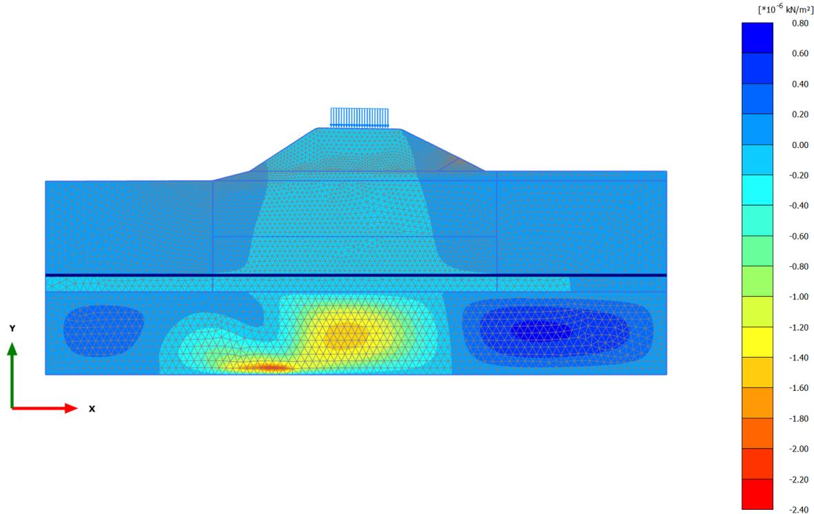
Excess pore pressures  $p_{\text{excess}}$  (scaled up  $1.00 \cdot 10^6$  times) (Pressure = negative) (Time  $36.83 \cdot 10^3$  day)
