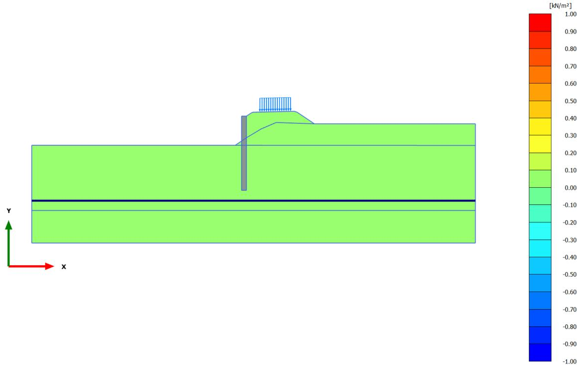
Excess pore pressures  $p_{\text{excess}}$  (scaled up  $500 \cdot 10^6$  times) (Pressure = negative) (Time  $36.83 \cdot 10^3$  day)
