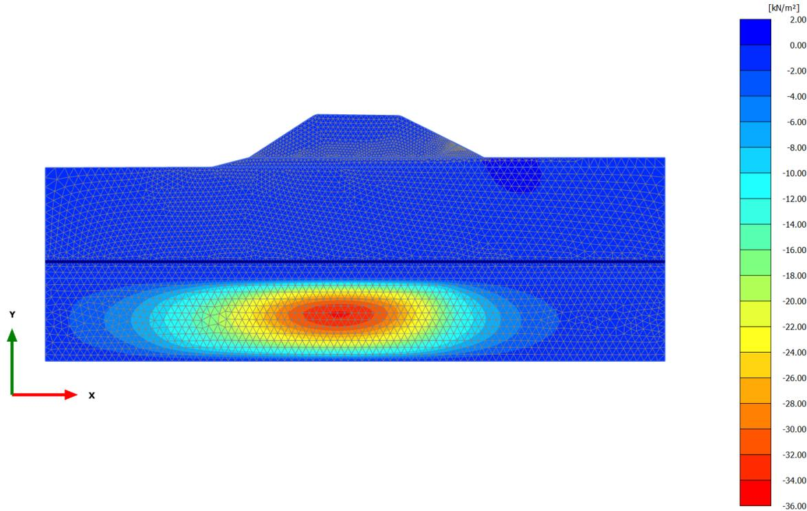
Excess pore pressures  $p_{excess}$  (scaled up 0.100 times) (Pressure = negative) (Time 330.0 day)
